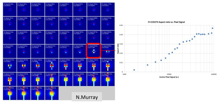
Point Spread Function intensity dependence, up to 10% effect on ellipticity
