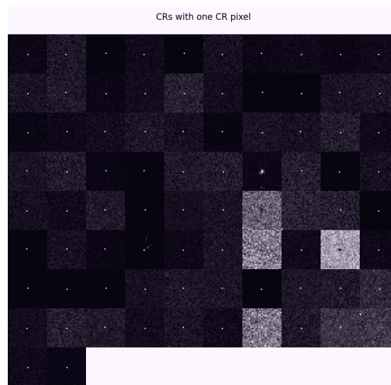
Figure 2: All of the examples of stamps with 1 pixel flagged as CR for visit 11710. It is clear that most of the stamps are in fact CRs so the cutoff=1 is chosen.
