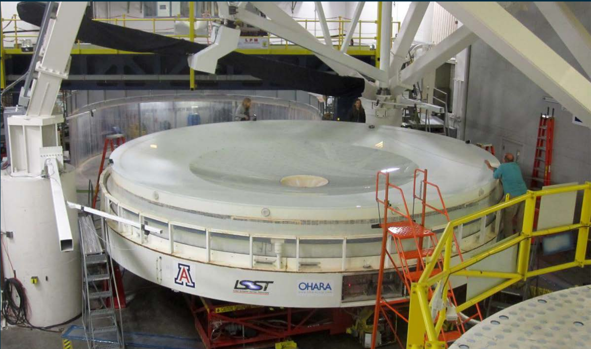
8.4m diam Primary with 5m diam Tertiary surfaces completed
